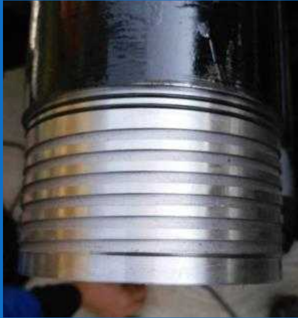
External flush pipe with O-ring seals
